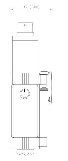
The Autozero function is activated through a magnetic contact (external magnet supplied with the sensor).
